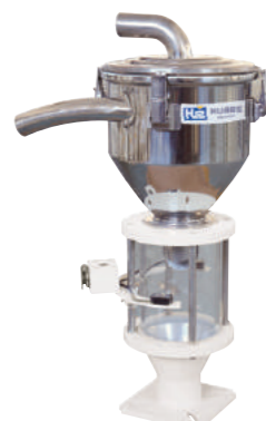
6升电眼料斗 / PH-6L 6L Photoelectric hopper
